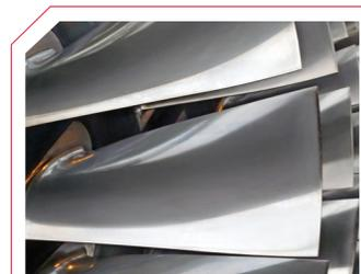
Figure 3: GT compressor blade with AAF HEPA (8,000 hours)
