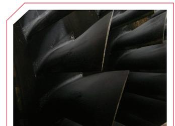
Figure 4: GT compressor blade without AAF HEPA (2,000 hours)
